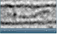
Transmission electron microscope video shows conformational changes in a carborane molecule bearing two alkyl chains that is confined inside a carbon nanotube 1.2 nm in diameter.
